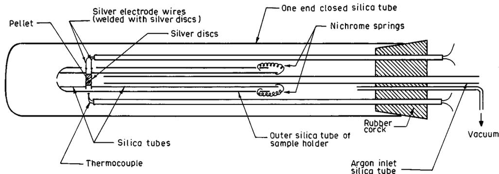
Figure 1 Schematic diagram of experimental cell assembly.
